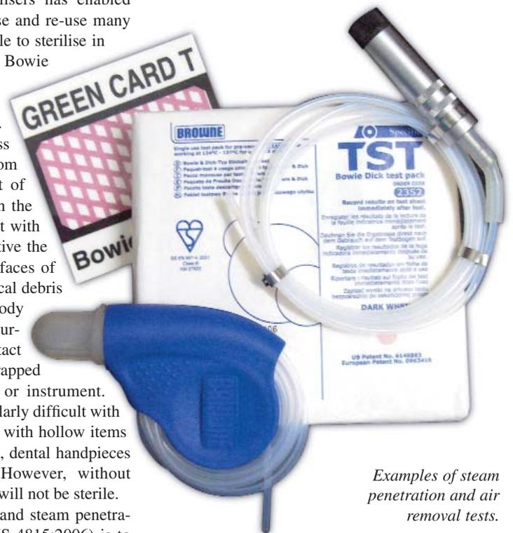
*Examples of steam penetration and air removal tests.*
