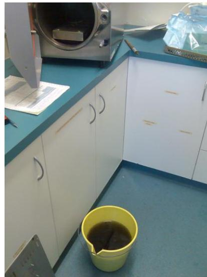
Fig 1: The water in the bucket has just been drained from the reservoir of the steriliser above and shows severe recycling contamination. The water in this steriliser had not been changed in six months. This is a common sight for technicians servicing sterilisers in busy practices.
