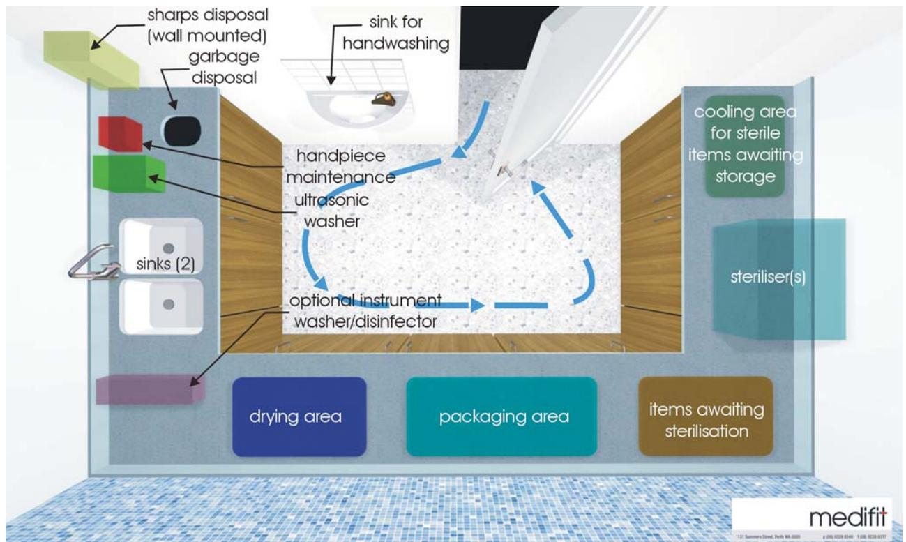
Figure 2. This shows the layout recommended for the correct flow (arrows) of instruments from dirty to clean to sterile in your reprocessing area. Existing areas can be modified to follow this as closely as possible (note: flow can be clockwise or anti-clockwise so long as it is in a single direction).
